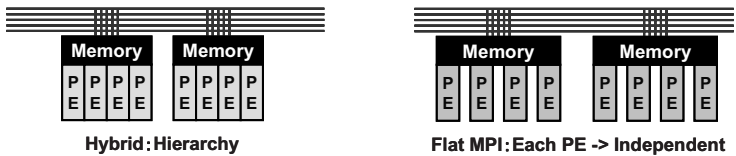
Fig. 1. Parallel programming models on SMP cluster architecture [1,2]
